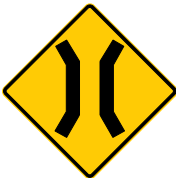
Narrow structure ahead — often a bridge
